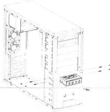
Placed in the floppy drive chassis position, lock fixed two screws on each side
